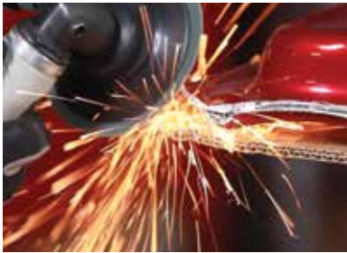
Door Skin Replacement
