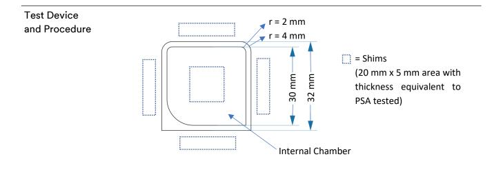
Due to the viscoelastic nature of PSA's, the applied pressure across the edge of simulated devices would be decreased due to the compression of the PSA. To account for this, it is necessary that samples would need to pass the same pressures, with and without, shims (at the same thickness as the PSA used) to maintain and compress the bond line, respectively. The simulated devices will be considered as passing the test when no visible liquid has entered the internal chamber of the device.
