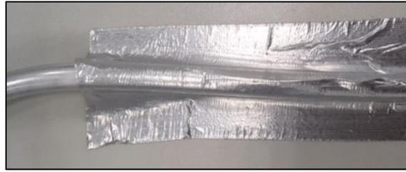
Figure 3: Tube attachment using aluminum tapes
