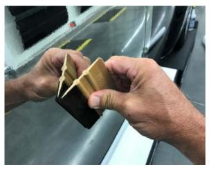
**Figure 3.** Use dampened, soft-sided squeegee for application. Always ensure the soft side is saturated with slip solution.
