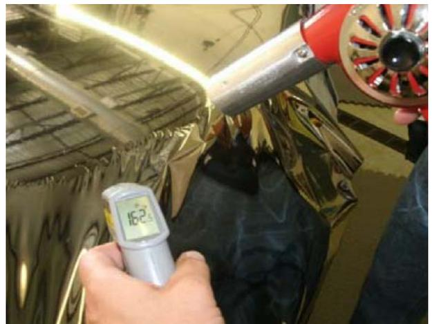
**Figure 2.** Heat the film to 150°F to 180°F (66°C to 82°C) and use an infrared thermometer to monitor the
