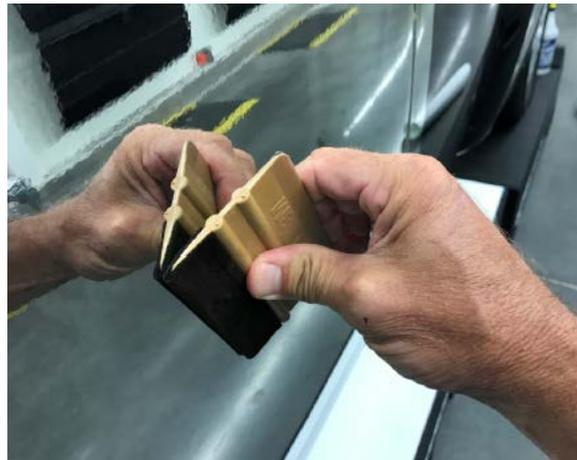
**Figure 3.** Use dampened, soft-sided squeegee for application. Always ensure the soft side is saturated with slip solution.
