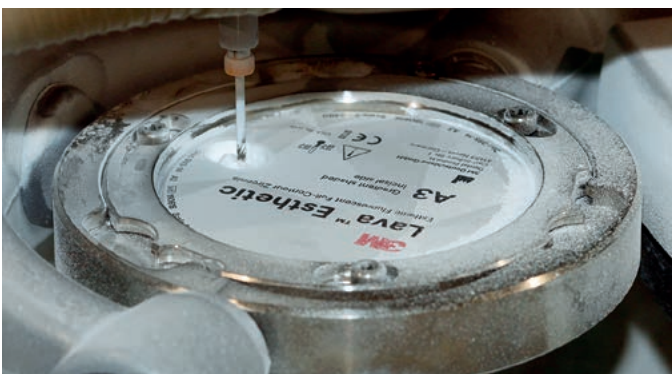
Milling of crown out of a 3M™ Lava™ Esthetic Zirconia A3 disc.
