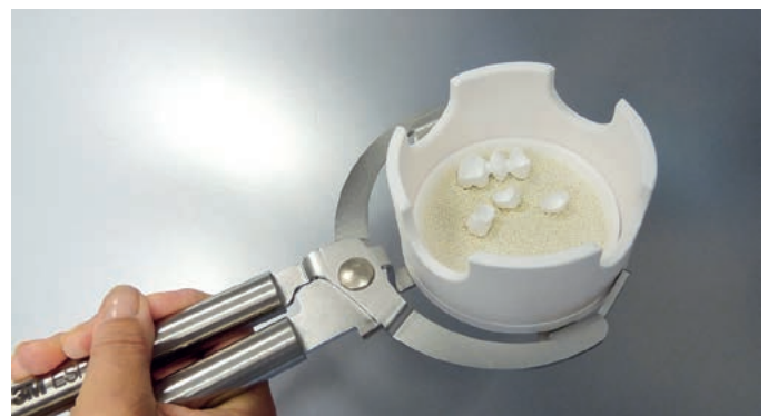
Sintering at 1500°C for 2 hours.
