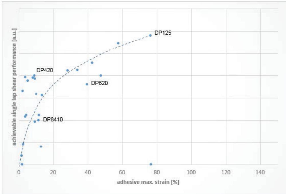
Figure 9: The above image shows the maximum achievable lap shear performance of a selection of adhesives on abraded glass-fibre-reinforced polyester substrates.
