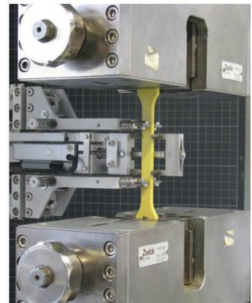
Figure 7: The image above is showing some stress-strain curves of a selection of adhesives. For this, load is applied to a dumbbell-shaped specimen as shown on the right side. The curves represent the different families of adhesives. Toughened epoxy (DP420), toughened polyurethane (DP620), methacrylate (DP8410), flexible Urethane (DP6330NS) and flexible epoxy (DP125)
