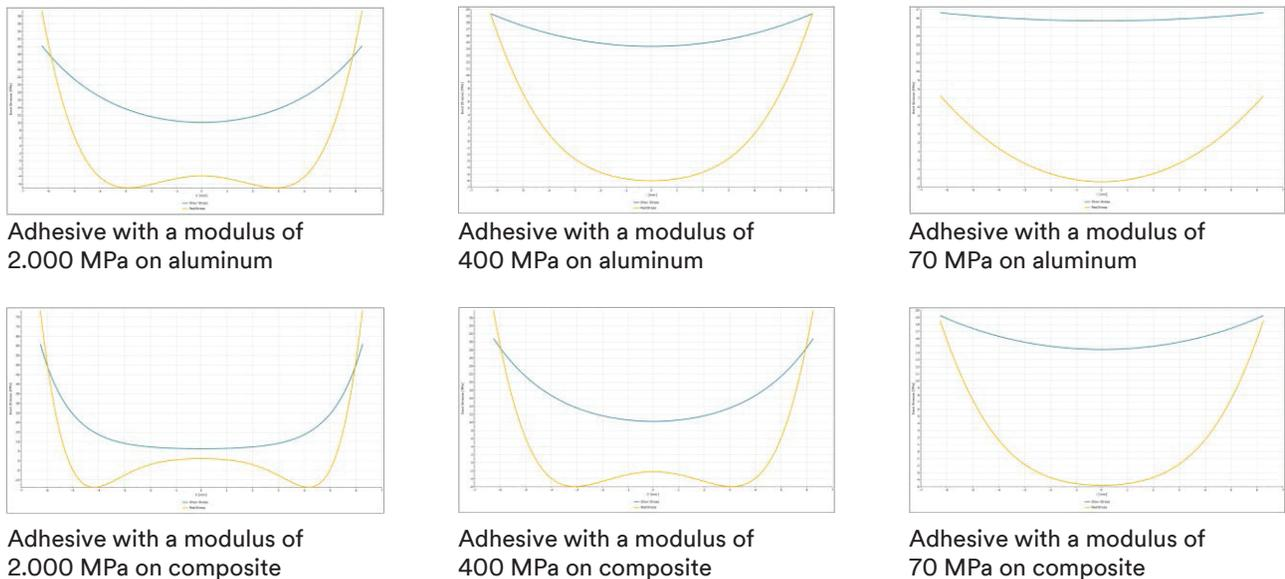
Figure 8: Closed form calculations of stress within an adhesive joint as a function of modulus of the substrates and adhesive.
