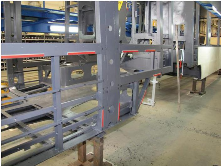
Figure 4. GRP panel bonding to steel using a 3M™ Adhesive Sealant
