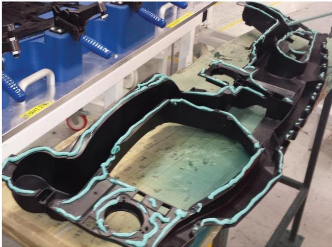
Figure 3. Lightweight glass-filled polyolefin bulk head moulding being bonded with 3M™ Scotch-Weld™ Structural Plastic Adhesive DP8010NS Blue to an aluminum frame
