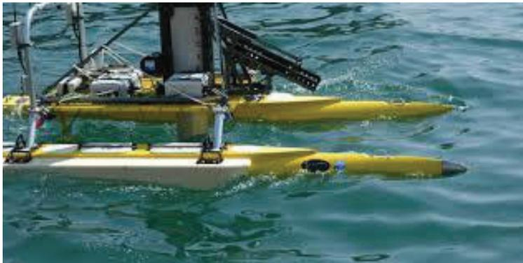
Figure 6. Syntactic foam buoyancy aid bonding to aluminum using a 3M™ Scotch-Weld™ Epoxy Adhesive 2216
