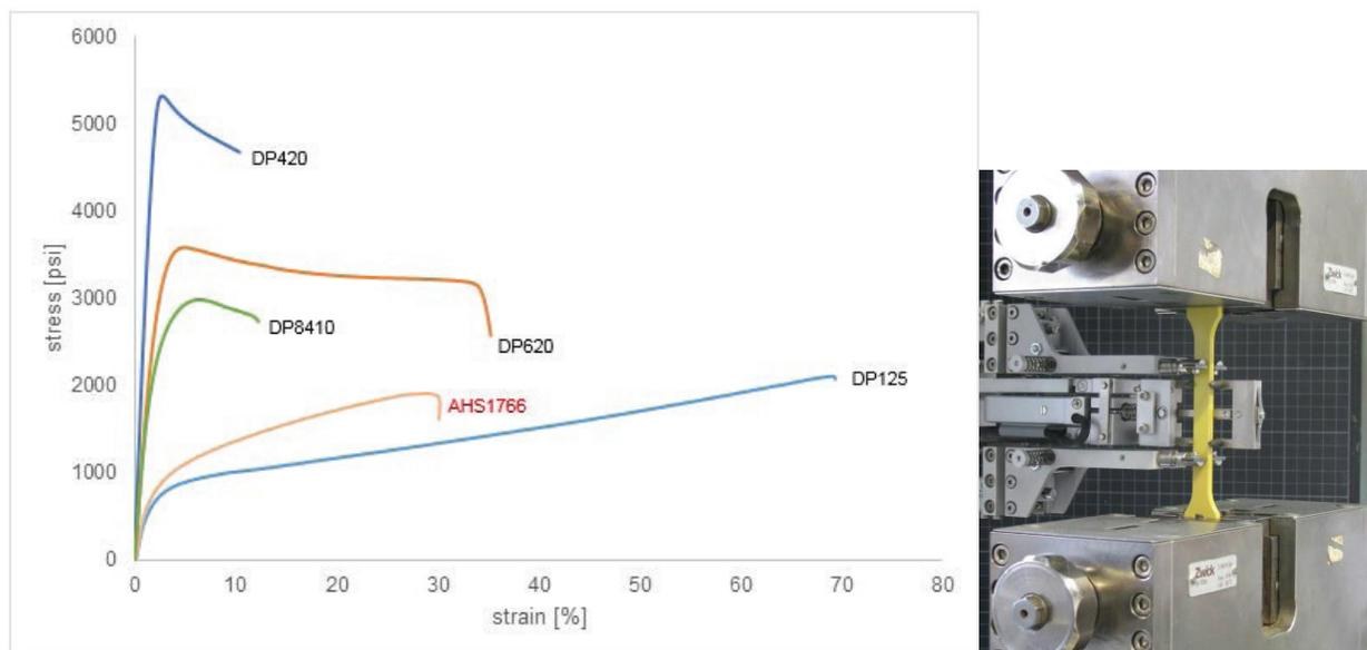
Figure 7: The image above is showing some stress-strain curves of a selection of adhesives. For this, load is applied to a dumbbell-shaped specimen as shown on the right side. The curves represent the different families of adhesives. Toughened epoxy (DP420), toughened polyurethane (DP620), methacrylate (DP8410), flexible Urethane (DP6330NS) and flexible epoxy (DP125)
