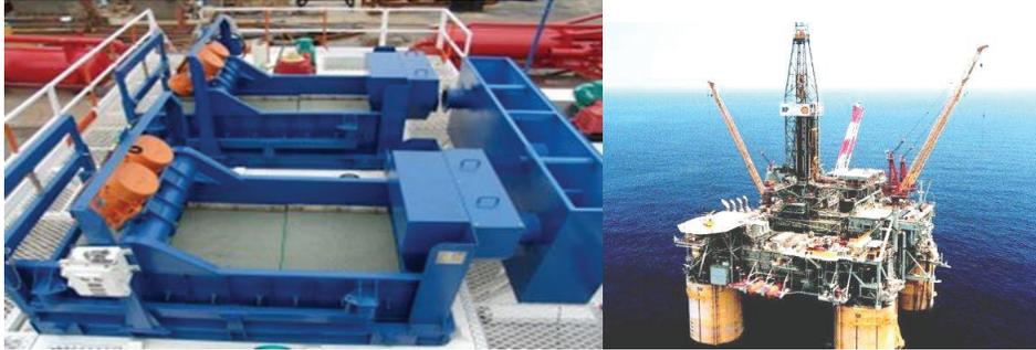
Figure 5. Carbon fibre composite panels bonded to stainless steel for lightweight oil shakers using a 3M™ Scotch-Weld™ Toughened Epoxy Adhesive.
