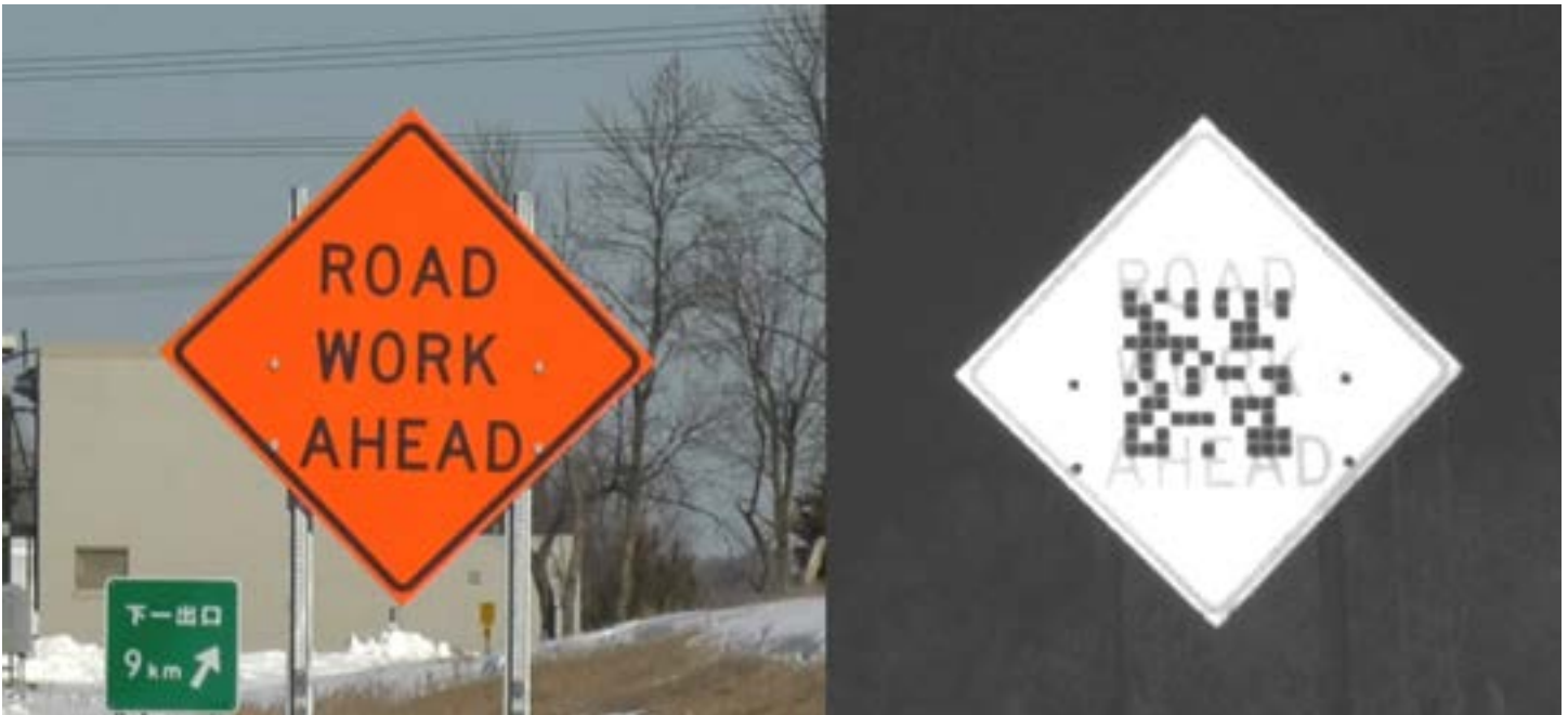
Figure 1: Visible and Near-IR View of 2D Bar Code
