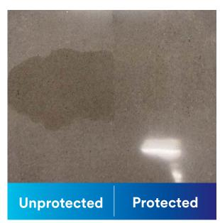
The above picture shows the stain left from exposure of concrete to motor oil with a 20 minute dwell time. Note the protected side resisted the motor oil while the unprotected side resulted in a stain.
