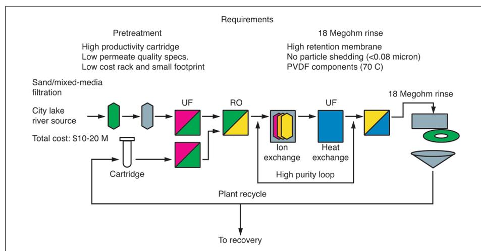
Figure 1: high-purity water production.
