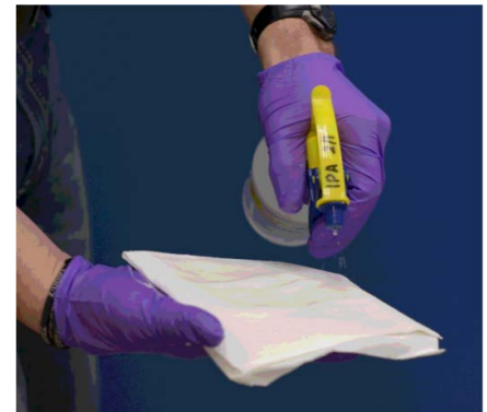
Figure 6. Soaking a Lint Free Cloth
