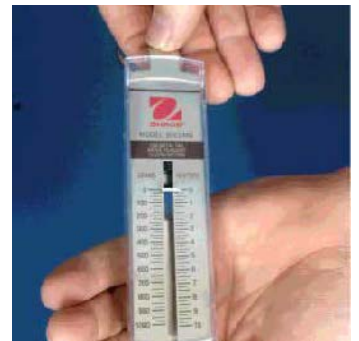
Figure 5. Zeroing the Scale
