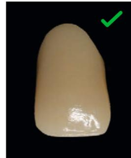
Control: 3M™ Lava™ Esthetic Zirconia crown, A3.5, glazed with e.max® Ceram Glaze Spray, firing temperature 770°C ▶ correct shade
