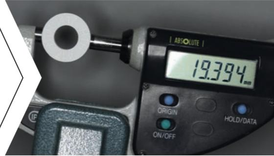
Compare ring diameter after sintering with diameter range provided by 3M for this ring lot. If the ring diameter is outside of the range, then furnace maintenance is recommended.
