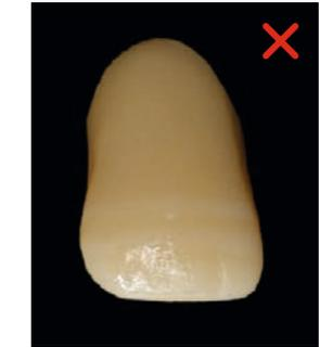
Over-sintered 3M™ Lava™ Esthetic Zirconia crown, A3.5, with decreased translucency, bleached shade and visible lines.
