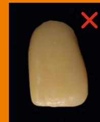
3M™ Lava™ Esthetic Zirconia crown, A3, glaze firing with lack of oxygen in the furnace ▶ yellow discoloration
