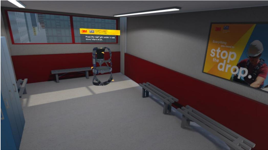
9. The User can conduct a visual inspection of the harness and simulate how to don the harness. This harness inspection is just a simulation, and in order to complete the inspection, the user must touch all six triangles on the harness as a way to inspect the harness.
