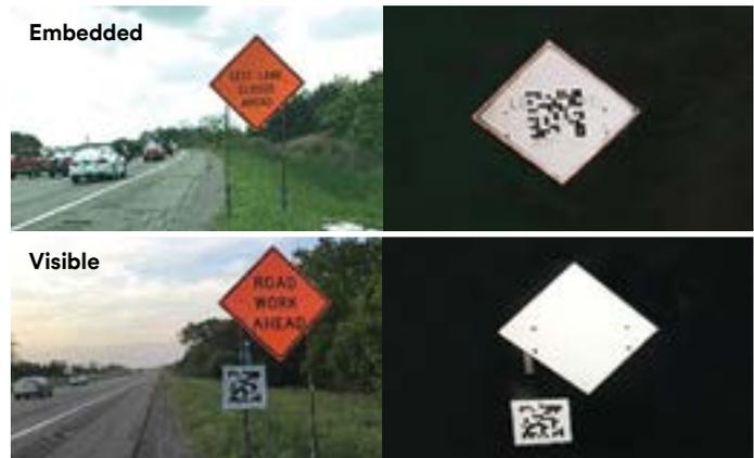
Signs with embedded and visible 2D barcodes were deployed to test the ability to provide information to automated vehicles at a variety of distances and under different circumstances.
