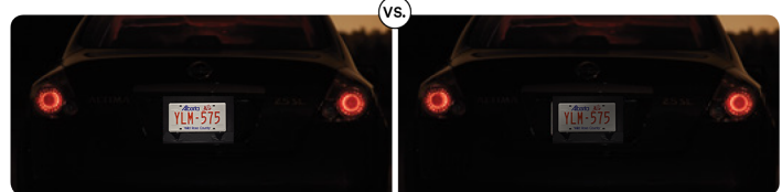
Legibility of 3M™ Series 6700 Sheeting at night vs. Traditional Beaded sheeting at shorter distances
