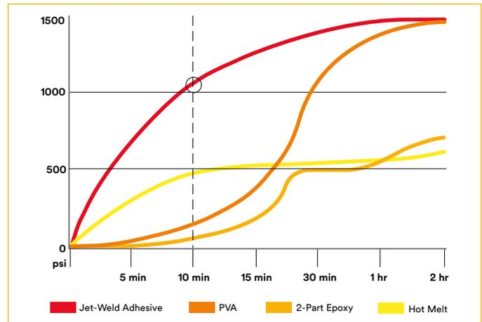
Jet-Weld Adhesive speed decreases fixture time to help increase productivity. In only 10 minutes, bond strength exceeds the structural strength base line of 1,000 psi in lap shear. After an hour, strength is greater than many substrates (note splice test below).
