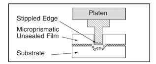
For a flat, continuous, linear weld, a tool width of approximately 2 mm is recommended. For this application, radiused/rounded tool edges are essential to ensure sideways displacement of the prisms. This allows for better contact between the 3M™ Scotchlite™ Reflective Material top film and the substrate.
