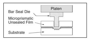
For applications where a wide weld area is required, a tool design incorporating stippled edges is effective. These provide spaces adjacent to the weld contact zones that enable prism displacement. Tools with radiused/rounded edges are recommended.
