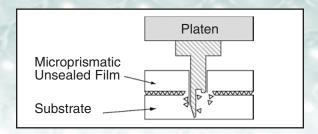
Note that the sealing flat should have radiused/rounded edges, again enabling sideways displacement of the prisms.
