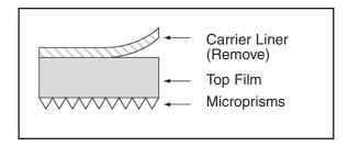
To use the product to achieve retroreflective properties, the microprism structures should face towards the article upon which this film is being applied. Conversely, the smooth surface should face outward.
