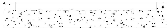
Figure 11. Cross sectional illustration of the texture of a groove made with a flail-head grinder-type cutting head.
