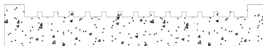
Figure 5. Cross sectional illustration of a coarse-tooth ribbed pattern produced by widely spaced or worn blades. Replace blades and/or change spacing to avoid such groove patterns.
