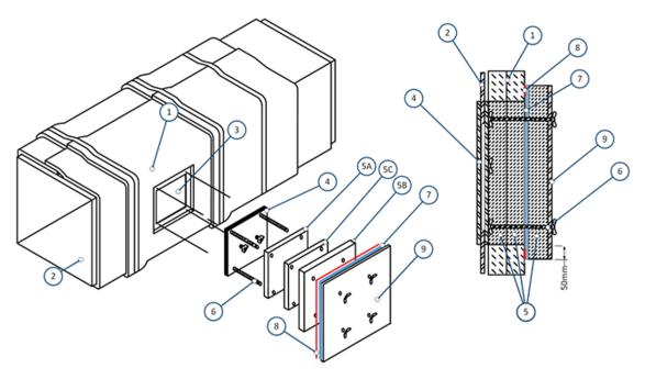
General Procedure Continued: Apply 3M Self Adhesive intumescent strip, with a minimum of 20mm width, to the perimeter of the plasterboard, with flush fitting mitre cut corner joints. Drill holes in the plasterboard that match the location of the four all-thread, steel rods and locate the holes so that the plasterboard is squared.
