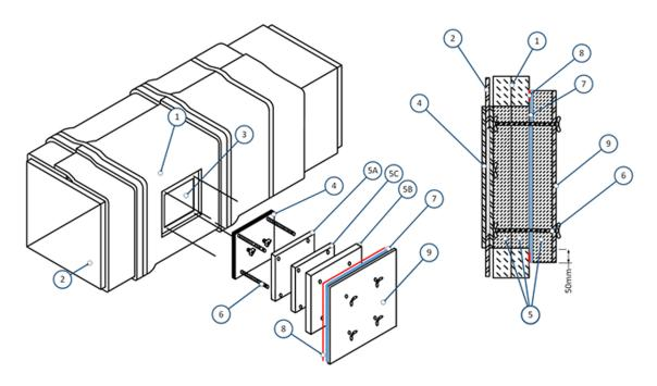
**General Procedure:** Cut hole in the duct using the template supplied with the pre-fabrication access door, and pre-install the door as per the access doors supplied instructions.
