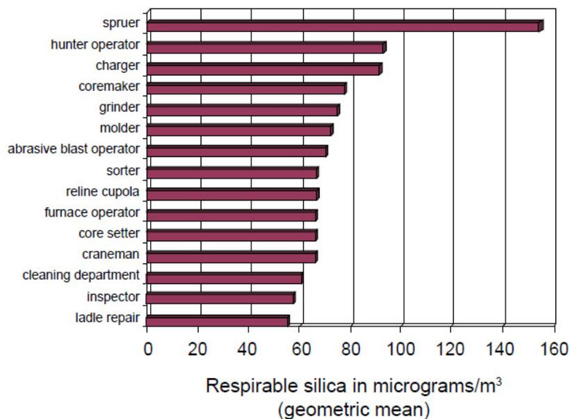
**Figure 1.** Crystalline silica exposure levels measured by the U.S. Occupational Safety and Health Administration (OSHA) for several foundry operations.<sup>1</sup>
