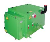
3M<sup>™</sup> Abators remove EO gas exhausted from 3M<sup>™</sup> Steri-Vac<sup>™</sup> Sterilizers/Aerators, catalytically converting exhausted EO into CO<sub>2</sub> and water vapor to meet environmental requirements. At normal operating temperatures and concentrations, removal efficiency is 99.9+% (when EO is >100 ppm).
