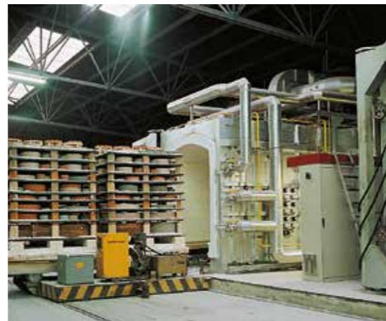
Kilns with electronic control of the temperature curve for reproducible and documented quality.
