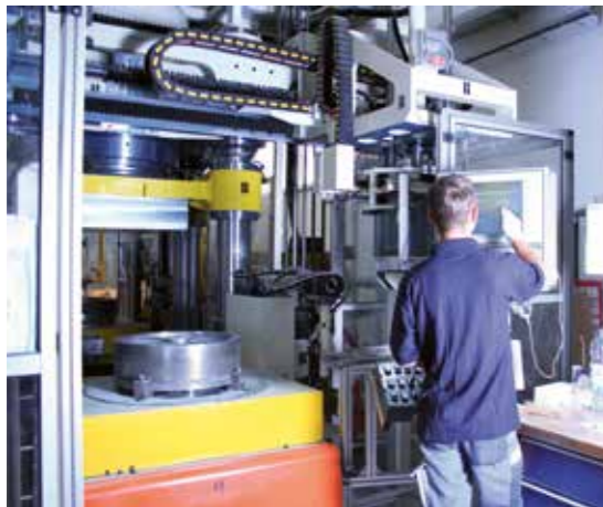
CNC-controlled presses to ensure the homogeneous wheel structure is reproducibly maintained.
