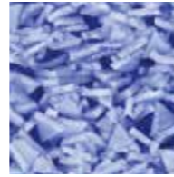
3M Precision-Shaped Grain (Sintered corundum)
