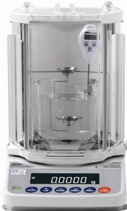
Figure 2-13. Archimedes density measurement set-up. Picture courtesy of A&D Weighing [32].
