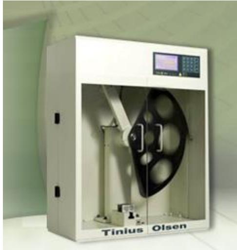
Figure 2-10. Picture of Tinus Olson Impact tester. Picture Courtesy of Tinus Olson [30].
