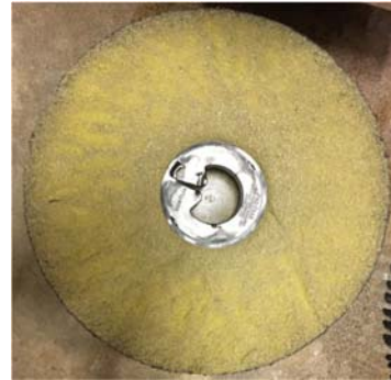
Flip pads after the first side has worn away. Discard after second side has reached end of life.
