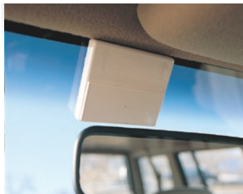
Mount transponder on windshield
