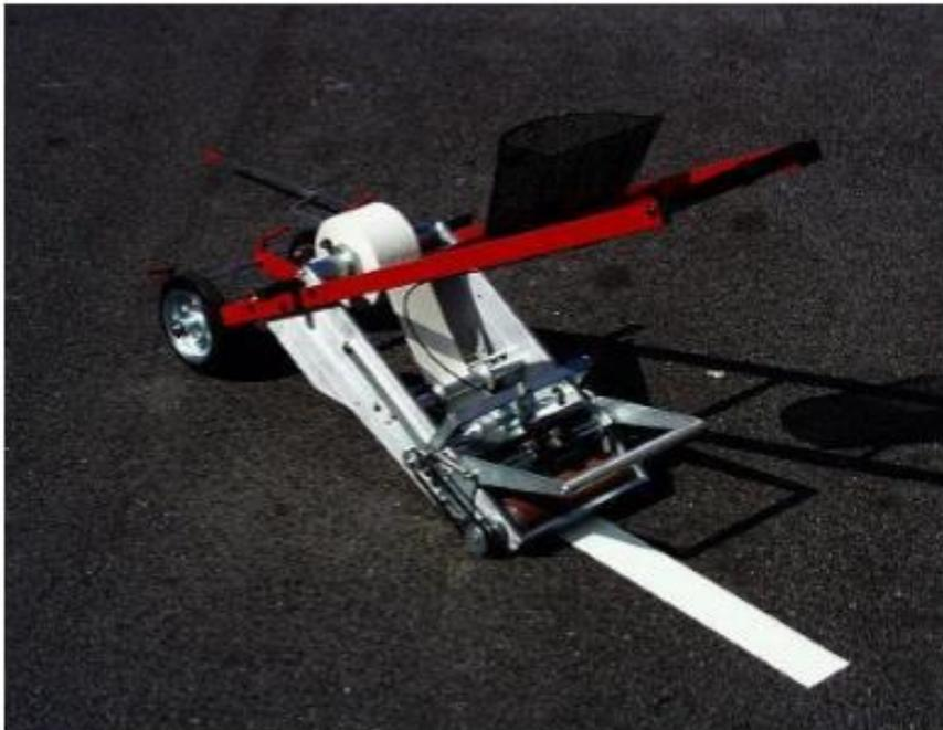
**Figure 1: MTA-2 Tape applicator**
