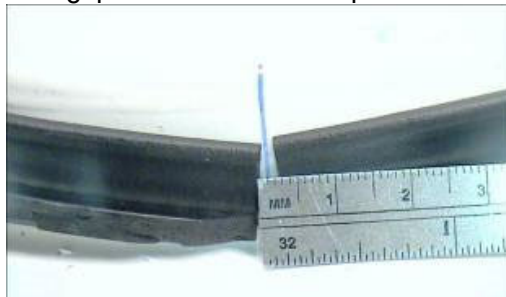
Seal has been cut and reapplied along original path; gap is measured with a ruler.
