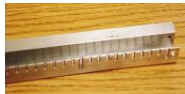
Close-up view of seal marking fixture. Deeper slits are made each 10cm, smaller slits are 1cm apart.
