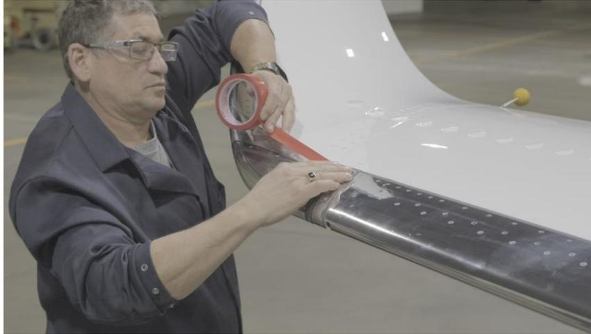
*Figure 1: Apply masking tape to enable neat edge seal application*
