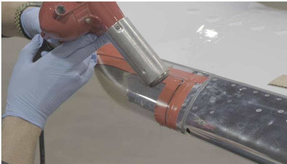
*Figure 4: Gentle heating can accelerate the edge seal cure*
