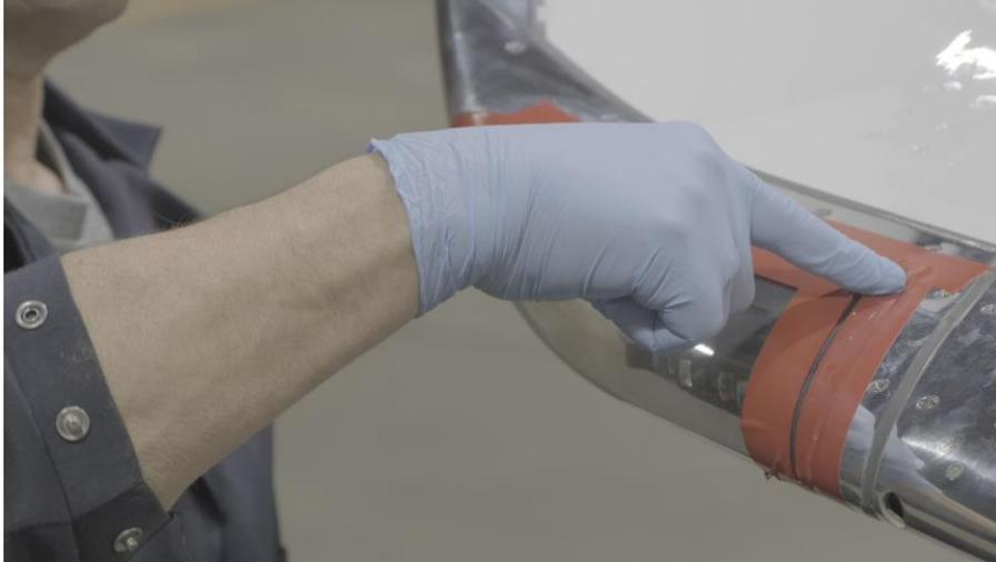
*Figure 3: Edge seal should be smoothed after application*
