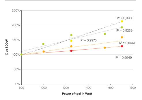
Looking at the cumulative effects, just by changing the MO, in theory life improvement of factor 25 could be attained at the least efficient working customers. Overall the 3M cut-off wheels proved to be rather robust. Cubitron™ II cut of wheel showed a maximum impact of slightly more than 6 times the life span.
