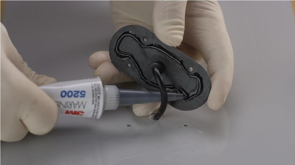
Figure 7: 3M 5200 Marine Adhesive Sealant provides the strength required to bond through-hull fittings and reliably seal below-waterline applications over the long term.
