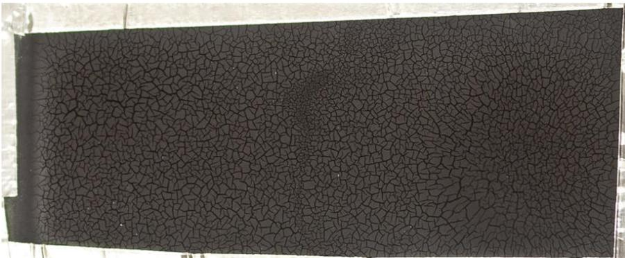
Figure 4: Seal is compromised and needs to be reapplied or replaced
