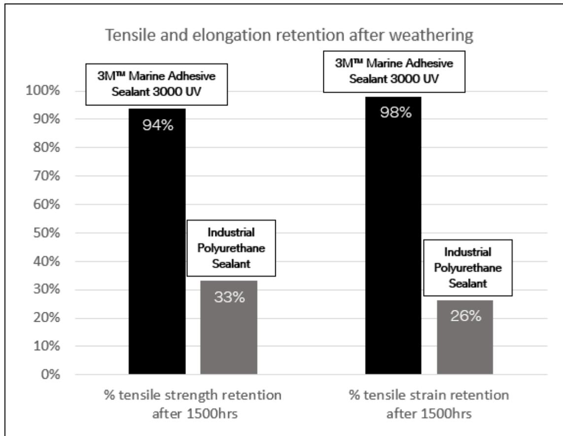
Figure 5: 3M scientists use data like this to determine what the issues are with a sealant, improve formulations and increase adhesive stability.
