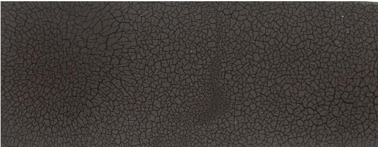
Figure 1: Cracks in the sealant can often be an indication of premature degradation.
