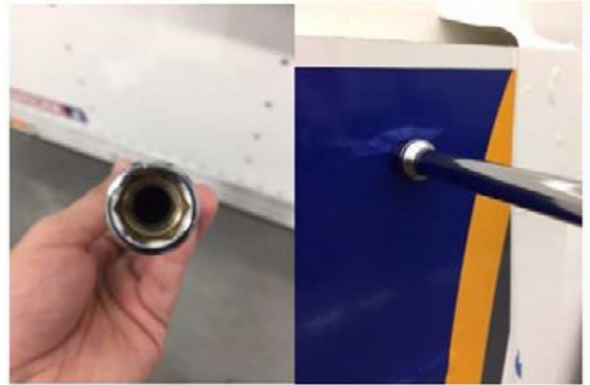
Figure 11. Using a circular-shaped tool to conform the film around a rivet
