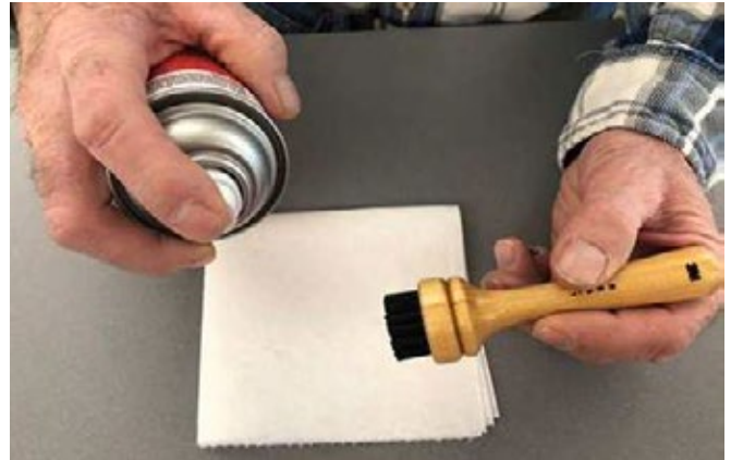
Figure 4. Applying silicone spray lubricant to the rivet brush
