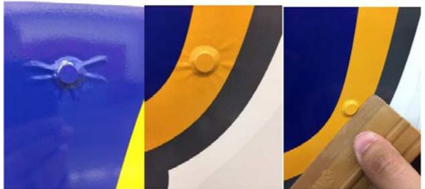
Figure 12. Conforming the film around a rivet
