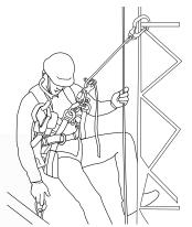
Connect the Trigger X Adjustable Rope Positioning Lanyard to a suspension D-ring or spreader bar (2108403) and attach the large snap hook to the anchor. ANSI and ASTM rated for single mode use.\*
