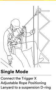
\*The rope adjuster meets ANSI Z359.3 and meets ASTM F887-13.
