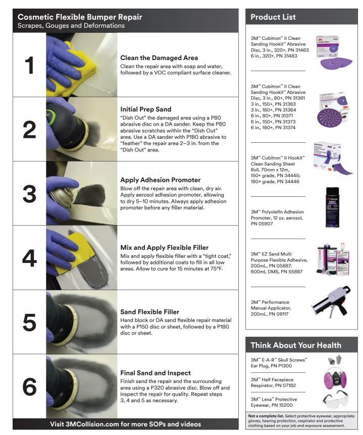
Note: We do not recommend a final coat of 3M<sup>™</sup> Polyolefin Adhesion Promoter (PN 05907) after the final sanding. The paint companies all recommend their own paint adhesion promoters and applying the PN 05907 may cause a compatibility issue.
