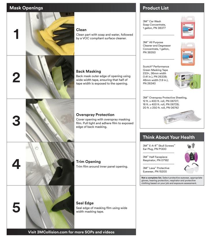
Note: All critical edge, jamb masking and general masking should be completed prior to masking openings.
