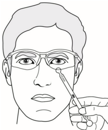
Figure 5B: Checking Gap
