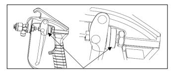
Figure 16: Trigger stop should always be fully closed when changing or modifying spray tips.
