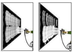
Figures 11-12: Maintain a constant speed while spraying that is delivering between 80-90% adhesive coverage.
