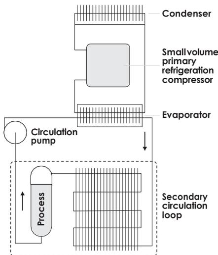
Novec fluids are ideal for heat transfer applications at low temperatures (down to -120°C). In this application, Novec engineered fluids are used in a secondary loop which transfers heat from the process to a primary refrigerant cycle. The unique set of properties (low freezing temperature, low viscosity and low surface tension) makes the Novec fluids easy to pump at very low temperature. The secondary loop works at low pressure, greatly reducing the risk of fluid loss.
