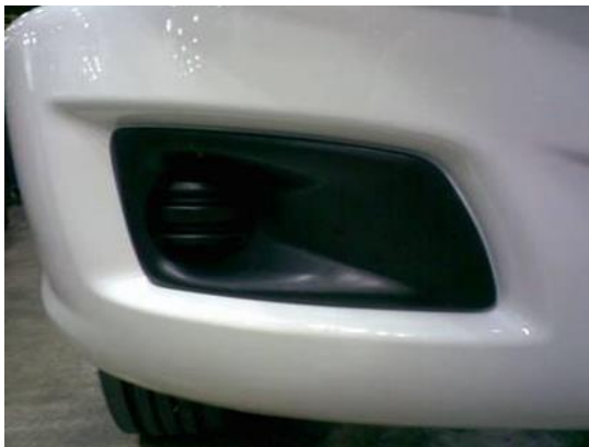
Figure 3 ABS to glass-filled polypropylene using 3M™ Scotch-Weld™ Structural Adhesive
