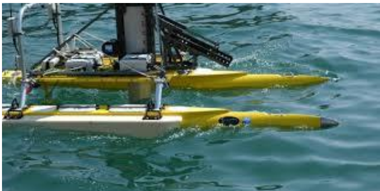
Figure 7. Syntactic foam buoyancy aid bonding to aluminum using a 3M™ Scotch-Weld™ Epoxy Adhesive 2216
