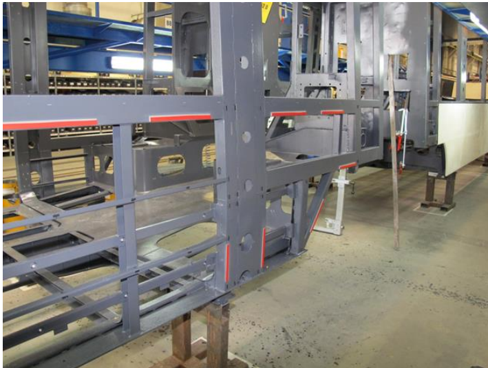
Figure 5. GRP panel bonding to steel using a 3M™ Adhesive Sealant
