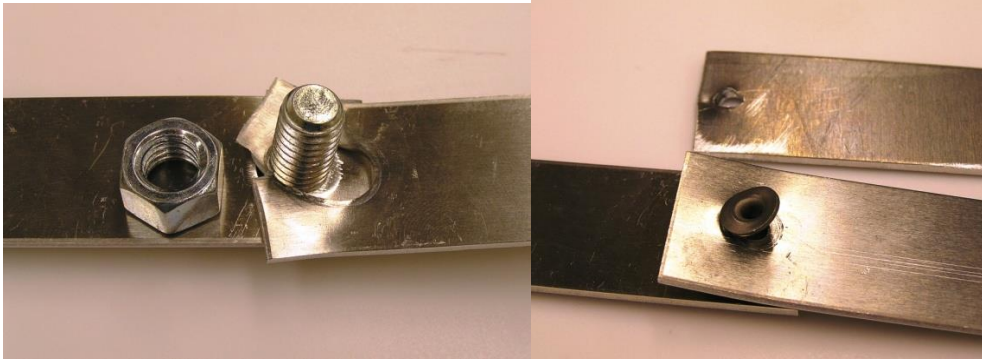
Figure 6. Failure of T6061 aluminum (0.063” thick) and rivets upon tensile force application vs. adhesively-bonded aluminum.
