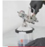
**5** Choose the right adapter for your spray gun. Push down and twist until adapter locks into lid. (Go to [3MCollision.ca/PPSAdapters](http://3MCollision.ca/PPSAdapters) to find the adapter that fits your spray gun.)
