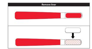
Remove release liner from brake insert (I).
