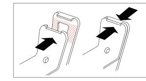
Slide the top of the wood deck (B) under the aluminum tooth of the aluminum base (A) until it snaps into place, and apply pressure.
