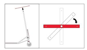
Insert the aluminum handlebar (H) parallel with the wheel (dowel pins up) and turn clockwise 90 degrees. 10
