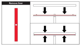
Remove release liner from the aluminum handlebar (H).
