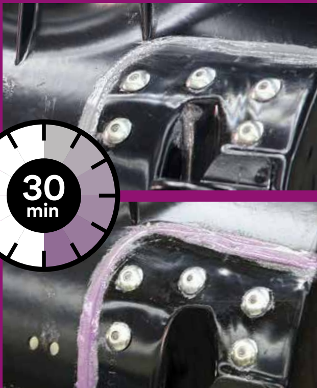
Cure indicated by silver to purple colour change (30 min at 80°C)
