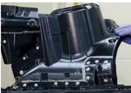
Adhesive bead starts silver in colour and changes to purple once curing is underway
