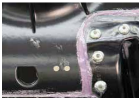
Cured product is purple to indicate proper mixing and complete cure
