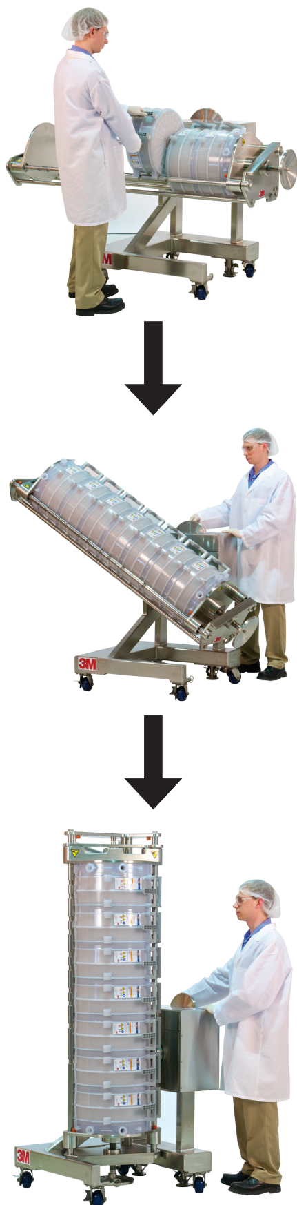
Figure 1: Zeta Plus™ Encapsulated large holder loading process
