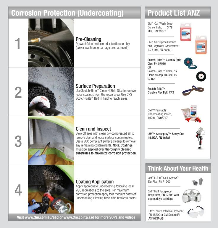
Note: Use caution when working on aluminium parts. Use tools that have been cleaned properly or designated for use on aluminium to reduce potential cross contamination. Do not re-use abrasives that were previously used on steel repairs.
