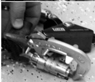
Figure 56 - Web or Rope Model, Attach Captive Eye Carabiner to Cynch-Lok Roller Adjuster
