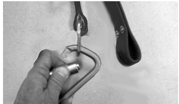
Figure 60 - Connect Body Support Carabiner to Web End
