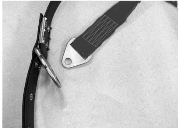
Figure 35 - Pull Web Lanyard through the Dual Slot D-Ring
