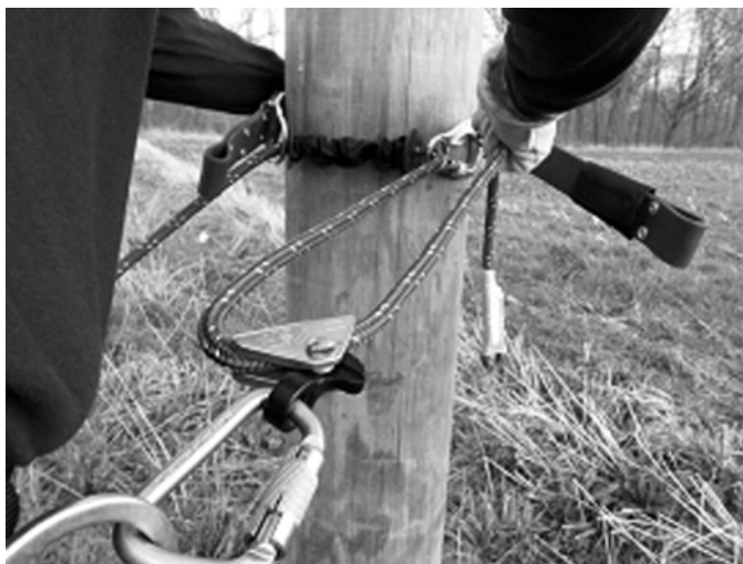
Figure 22 - Adjust Out from Pole, Web Version
