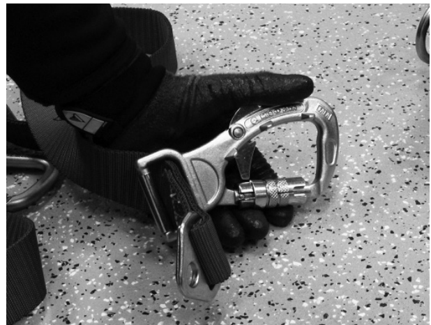
Figure 55 - Insert Web Lanyard into Captive Eye Carabiner (Model 1204077)
