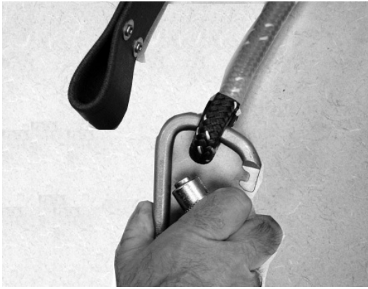
Figure 39 - Connect Body Support Carabiner to Rope Lanyard
