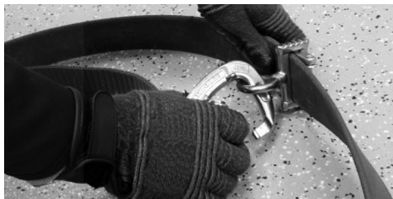
Figure 56 - Web or Rope Model, Attach Captive Eye Carabiner to Cynch-Lok Roller Adjuster
