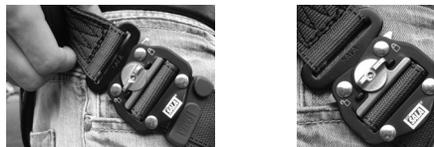
**Strap Adjustment:** Rotate Webbing Lock to unlocked position **B**. Pull strap to adjust. Rotate Webbing Lock to locked position **A**.
