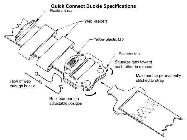
**<u>Buckle Operation</u>**: The quick connect buckle consists of two parts. The male portion is a metal tongue with flanges on the end. This portion is permanently attached to the end of a strap. The joining strap is woven
