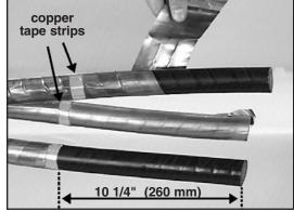
2.5 Remove cable semi-conductive insulation shields from conductors of both **Cable X** and **Cable Y** a distance of 7 1/4" (184 mm) from the end of each conductor.
