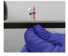
**C.** Ensure that the screw in the end cap removal tool is inserted all the way into the hole so the screw head is flat against the bar.
