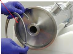
F. Install the retaining ring Clips by setting them into the holes in the end cap.
