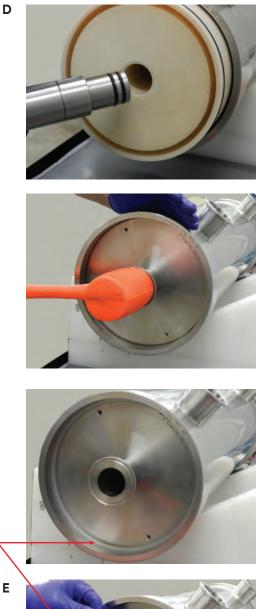
Groove on inside of vessel
