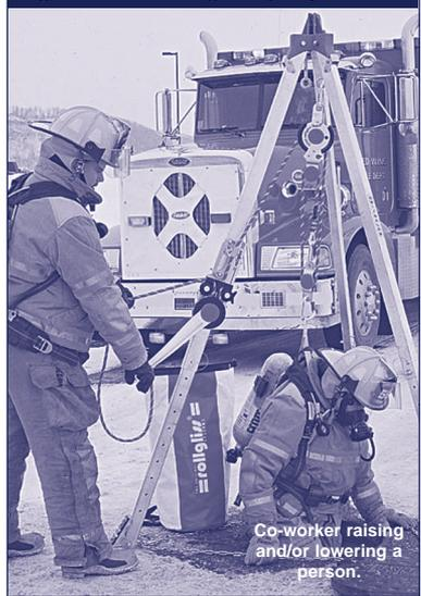
restricted to only a few feet when a 3:1 or 4:1 ratio is used. The maximum length of rope available for the system is 1500 feet.
