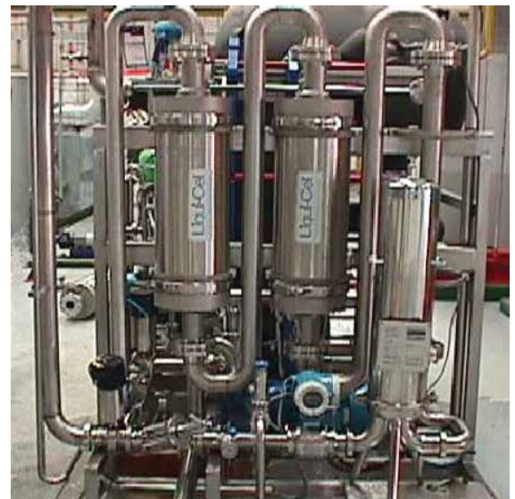
10 × 28-inch 3M™ Liqui-Cel™ Membrane Contactor Deoxygenation System
