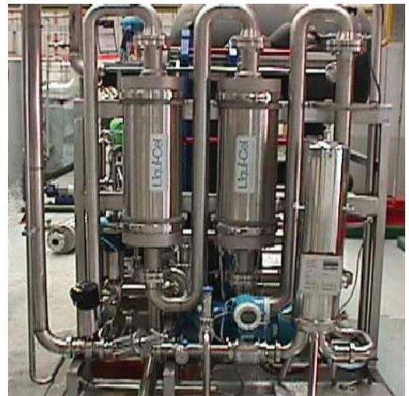
10 × 28-inch 3M™ Liqui-Cel™ Membrane Contactor Deoxygenation System
